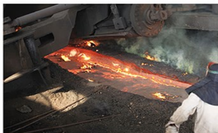
使用后期铁沟（单铁口小高炉） Late stage of iron trough (single iron of mouthsmall blast furnace)
