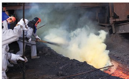
铁沟热态喷注修补 Hot shotcreting repair of iron trough
